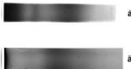
Fig. 5. The Guinier pattern of two EB-I samples. The beams are monochromatic ( \text{CuK}\alpha ): (a) X-ray pattern of the same sample as ä; (b) X-ray pattern of the same sample as ä; this figure shows clearly small angle scattering with pre-peak.
